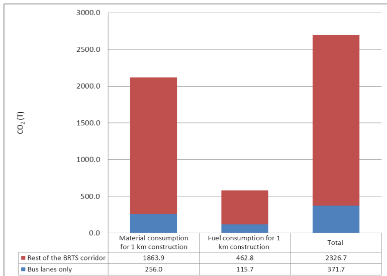
Figure 5.9 BRTS - Embodied CO 2 (tonnes) per km construction
